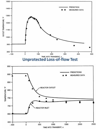
Unprotected Loss-of-heat-sink Test
